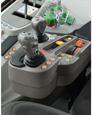
The RVshift transmission on the Lamborghini Spark R Stage V also has two settings [Normal and Heavy Duty] to optimise the draft force according to the job being carried out. In all speeds from 1st to 15th, the transmission can switch between ranges in response to tractor load. The Heavy Duty range can also be selected manually from a dedicated control on the right hand console in the cab.
