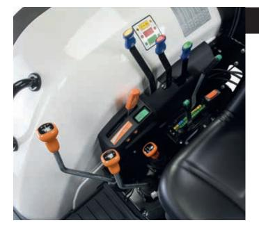
Hydraulic and Lift configurations are no exception when it comes to your working needs with 2 options of hydraulic capacity in the form of either 48 or 56 l/min, and auxiliary distributors from 2 to 6 ways with flow regulation. In addition all models feature an independent pump feeding the steering system only.
